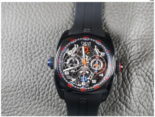
The movement, the Calibre CYR718, features two colour-coded column wheels which correspond to the respective colour-coded, crown-based circlet. The crown at 3 o'clock (see red circlet) engages with the red column wheel at 12 o'clock. Likewise, the crown at 9 o'clock (see blue circlet) converses with the blue column wheel at 6 o'clock.
