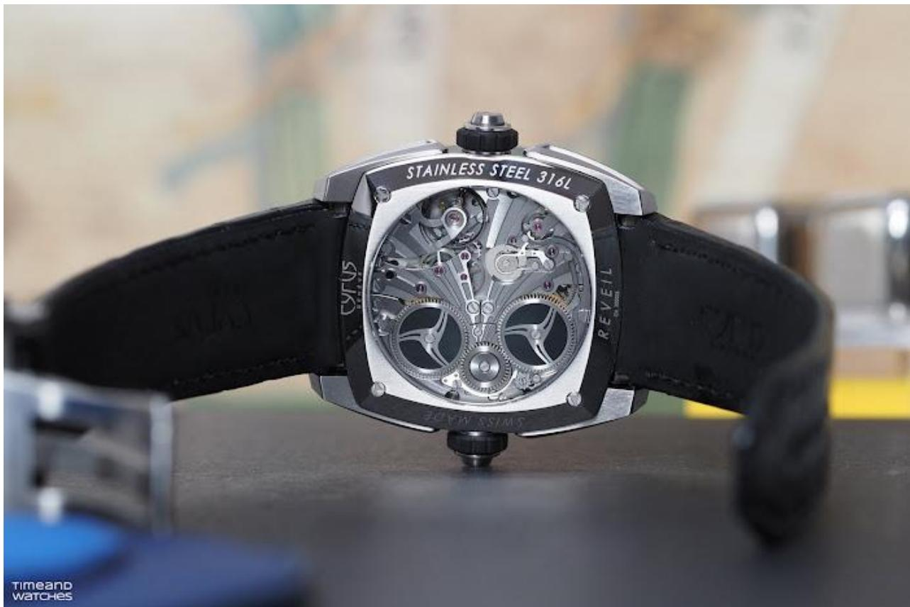
Comprising 340 individual components, this sophisticated movement operates at a frequency of 4 Hz (28,800 vibrations per hour) and provides a substantial 72-hour power reserve.
